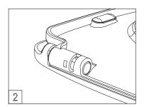
4) Put the buckle onto the buckle hole, use a hammer to knock it slightly until it is locked tightly, and then finish the assembling.
