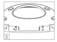
3) Assemble left soft-close set, set small hole and wide side rib upward and then push it into the cover.
