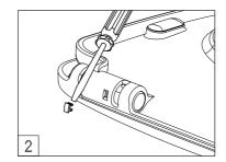
1) Use screwdriver, knife or any similar sharp tool to take out the buckle.
