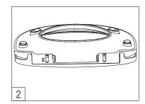
2) Assemble right soft-close set, set small hole and wide side rib upward and then push it into the cover.
