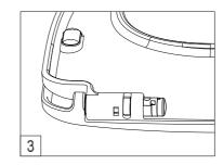
2) Use screwdriver, knife or any similar sharp tool to push soft-close set towards the right side, until expose the small hole on the press button, stick the hole and then push it towards right side until can not move further.
