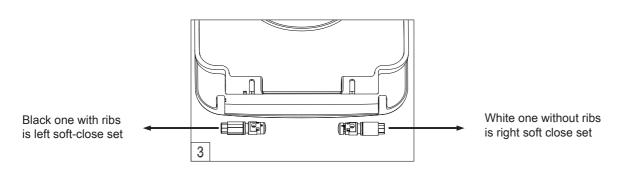
3) Lift up the left side of the seat slightly (Don't use too much power to avoid damage of S&C, lift it up to the point the seat can leave the cover. ), and then pull out the seat towards the left side to finish the disassembling.
