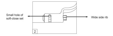
1) Put left and right soft-close set into the seat, make sure the small hole of the soft-close set and the wide side rib is upward.
